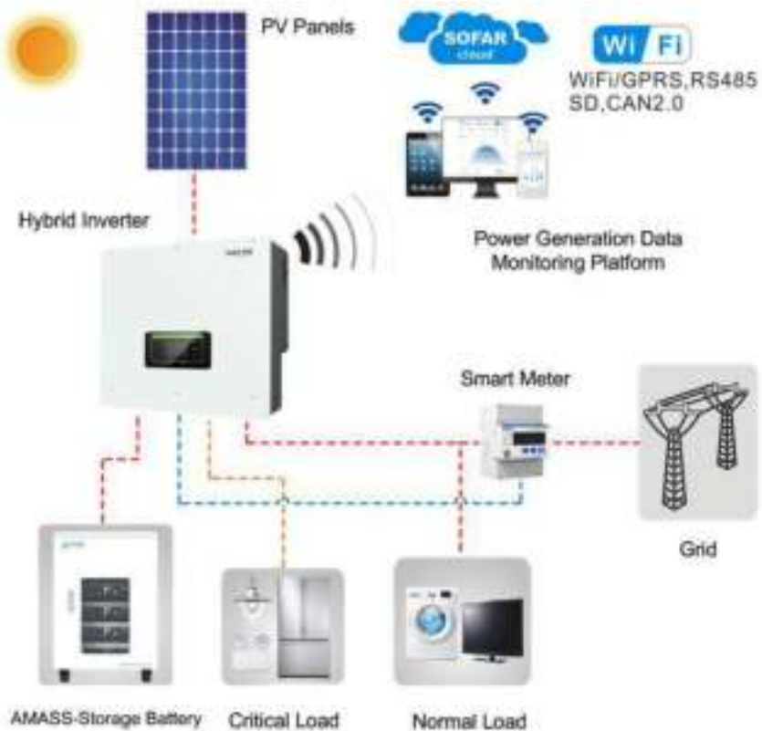
Fig. 3-1 Typical Energy Storage System
