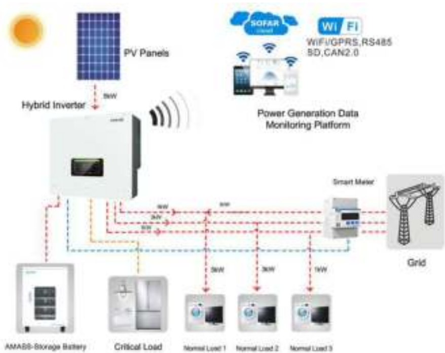
Fig. 3-9 On-Grid Unbalanced Output
