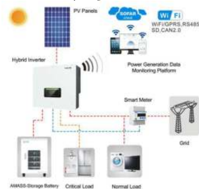
Fig. 2-1 HYD 5-20KTL-3PH inverter system diagram
