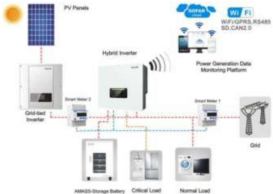
Fig. 3-7 AC Retrofit System(2)
