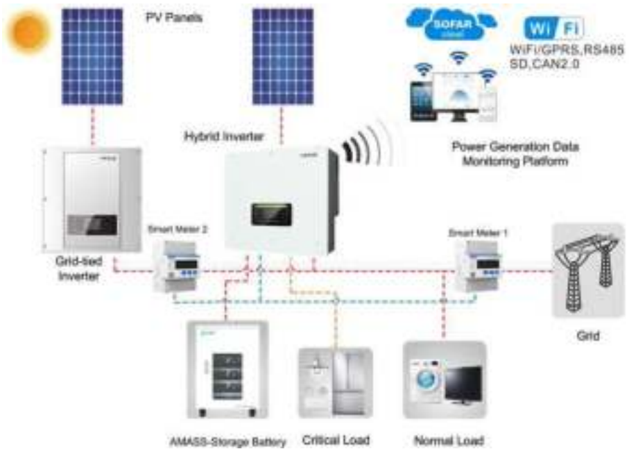
Fig. 3-6 AC Retrofit System(1)
