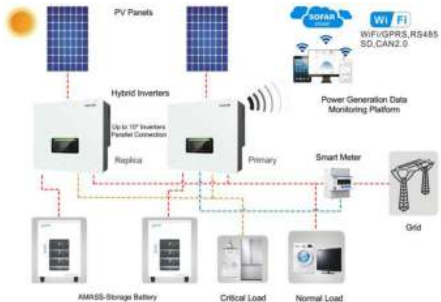
Fig. 3-5 System With Multi Inverters
