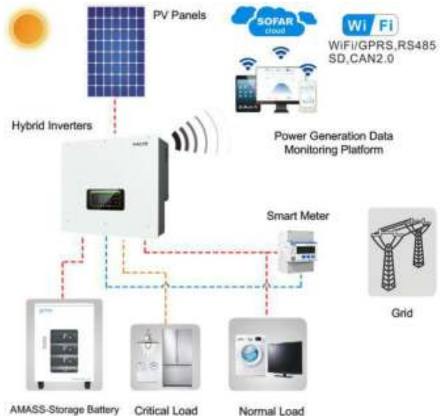
Fig. 3-4 Back-up Mode (Without Grid)
